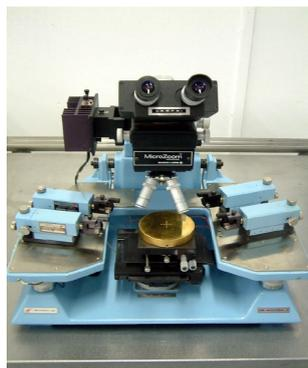
*Figure 4 Probe Station (Wentworth labs)*
